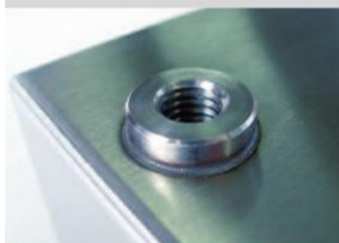
Circular welding at stainless steel housing (Photo: HAKAMA AG, Switzerland)
