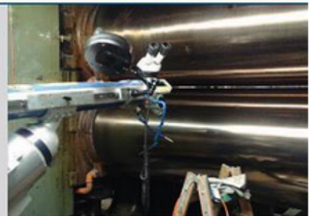
Repair welding on roller (Photo: tcms, Gummersbach)
