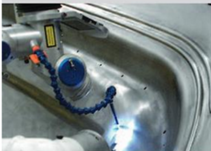
Repair welding (Photo: PML Lasertechnik, Nohra)
